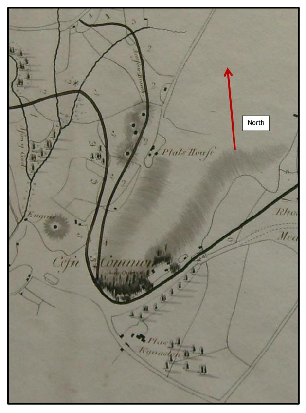
This extract is taken from the "Deviation of the Ellesmere Canal from Pontcysyllte to Chester with the Acrefair Coal and Holt Branches, Deposited 25<sup>th</sup> September 1795." It shows the Cefn Common on the ridge of what was also called the Cape of Kynaston and the start of the stone quarries that the Pontcysyllte Aqueduct would be carved from.
